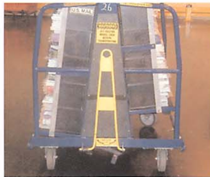
The newer spring-loaded tow bar was designed to eliminate bending and lifting the detachable tow bar.
