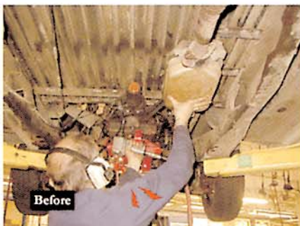
Before - In the Vehicle Maintenance Facility (VMF), mechanics often work with their arms overhead, such as here to hold the catalytic converter in place.
