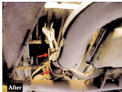
After - The mechanics connected a hook to a vise grip to hold the catalytic converter in place and enable the mechanic to reduce the time needed to accomplish the task.
