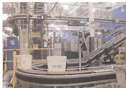
The Tray Management System eliminates much manual lifting. Among other features, trays are delivered at waist height (above right).
